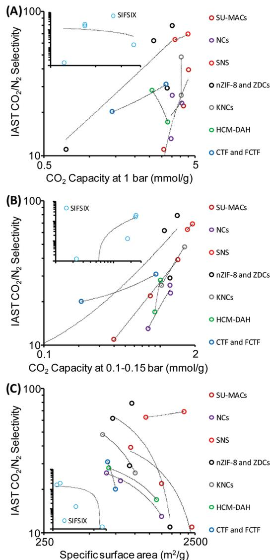
Fig. 10 Graphical “data mining” of the data shown in Table 1. CO<sub>2</sub>/N<sub>2</sub> selectivities (IAST or initial slope method) plotted versus (A) CO<sub>2</sub> capacity at 1 bar, (B) CO<sub>2</sub> capacity at 0.1–0.15 bar, and (C) specific surface area of the adsorbents. SIFSIX samples are shown in the insets for comparison.
