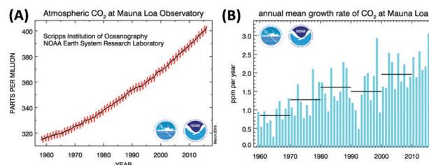
Fig. 1 (A) Increase of the atmospheric CO<sub>2</sub> concentration measured during 1958–2015 at the Mauna Loa (Hawaii). The red curve shows seasonal fluctuations, the black curve represents seasonally corrected data. (B) Annual mean carbon dioxide concentration growth rates. Decadal averages of the growth rate are also plotted as horizontal black lines.<sup>6</sup>
