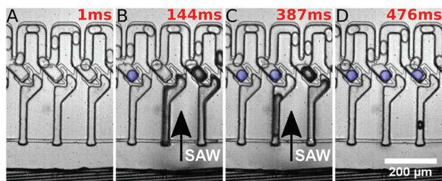
**Fig. 2** SAW induced trapping of droplets. (A) No droplet enters the trap when no SAW is applied. (B) A SAW pulse at a specific position, controlled by the applied frequency, is injected. The SAW hits the coupling channel and a bubble is generated at this location. (C) When the SAW is shut off, the bubble collapses and droplets (marked blue) are loaded into the traps. Successive droplets are passing by the already loaded traps. A pulse length of 350 ms and a pulse power of 29 dBm were used.
