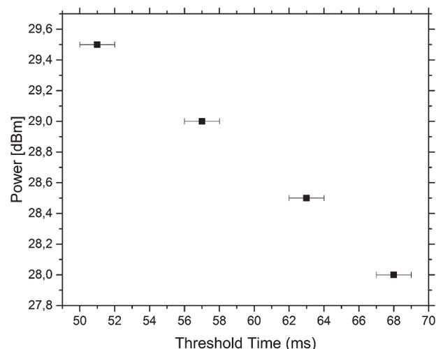
**Fig. 5** Power and threshold pulse length needed to push out a droplet. The third trap, being the middle trap, was monitored to measure the minimum time needed to push out a trapped droplet. The threshold time needed to push out increased with the decreasing power of the SAW.
