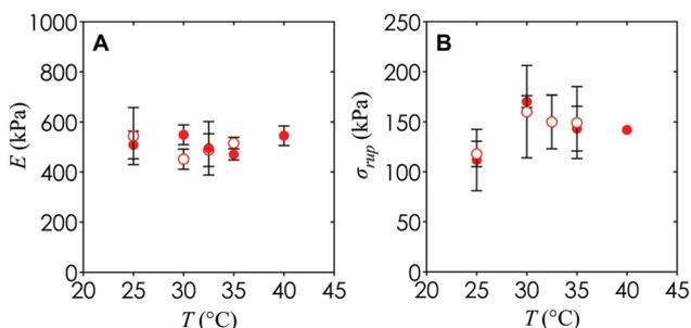
Fig. 9 Mechanical properties of filled and porous hydrogel scaffolds. (A) Young's modulus and (B) engineering rupture stress of the filled (solid) and porous (open) as a function of  $T$ . Error bars are standard deviations from 6 independent samples.
