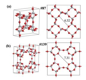
Fig. 6 Two new porous  ${\rm TiO_2}$  phases identified from the SSW-NN global search. (a) Phase-87; (b) phase-139. The Bravais lattices are shown on the left and the pore geometries with the pore size labeled are shown on the right.
