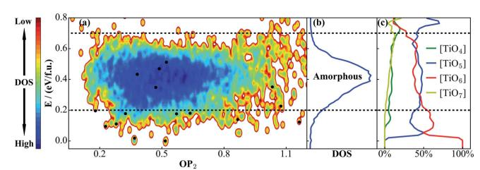
Fig. 5 (a) PES contour plot for  $TiO_2$  distinct minima sampled from the SSW-NN global search. (b) Density of states (DOS) plot for  $TiO_2$  phases in (a), showing that amorphous structures appear in the 0.2–0.7 eV f.u.<sup>-1</sup> window. (c) The percentage of differently coordinated Ti for  $TiO_2$  structures. [ $TiO_5$ ] and [ $TiO_6$ ] are the main structural features for amorphous structures. Also see the Fig. 2 caption for the meaning of the black dots
