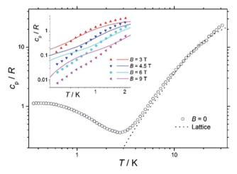
Fig. 7 Temperature dependence of the zero-field heat capacity  $c_{\rm p}$ , normalised to the gas constant R, for a polycrystalline sample of 1. The dotted line is the lattice contribution. Inset: temperature dependence of  $c_{\rm p}/R$  of 1 for T < 2 K and  $B \ge 3$  T. Solid lines are the best-fit curves, see text for details.
