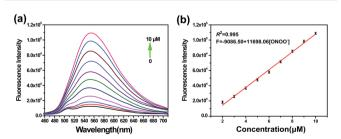
Fig. 2 (a) Fluorescence response of TP-KA (1  $\mu$ M) to ONOO $^-$  (0–10  $\mu$ M) in PBS buffer (50 mM, pH 7.4) with 1% DMSO. (b) The linear curve derived from the fluorescence intensity at 560 nm and the ONOO $^-$  concentration. The spectra were recorded after the incubation of TP-KA with ONOO $^-$  for 10 min at 37 °C. The values are the mean  $\pm$  s.d. for n=3.  $\lambda_{\rm ex}/\lambda_{\rm em}=430/560$  nm.
