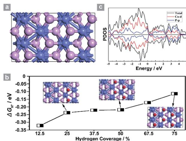
Fig. 4 (a) Simulated structure and (b) the dependence of  $\Delta G_{H^*}$  on hydrogen coverage  $\theta_{H^*}$ . (c) Projected density of states of the P terminated CoP (100) facet. Co atoms: blue, P atoms: purple and hydrogen atoms: red.
