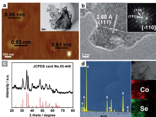
Fig. 5 (a) AFM image and TEM image (inset a), and (b) HRTEM images and the associated FFT pattern (inset b) of  $\text{CoSe}_2$  UPNSs. (c) XRD pattern, (d) EDS spectrum and STEM-EDS elemental mapping images (inset d) of  $\text{CoSe}_2$  UPNSs.
