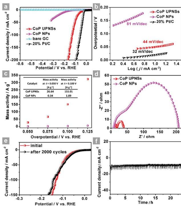
Fig. 2 (a)  $I$ - $R$  corrected polarization curves of CoP UPNSs, CoP NPs, bare GC and 20% Pt/C and (b) corresponding Tafel plots of CoP UPNSs, CoP NPs and 20% Pt/C in  $0.5 \text{ M H}_2\text{SO}_4$  at a scan rate of  $2 \text{ mV s}^{-1}$ . (c) Mass activity as a function of the overpotential for CoP UPNSs and NPs. (d) Electrochemical impedance spectra of CoP UPNSs and NPs. (e) Polarization curves of CoP UPNSs initially and after 2000 CV scans. (f) Time-dependent current density curve.
