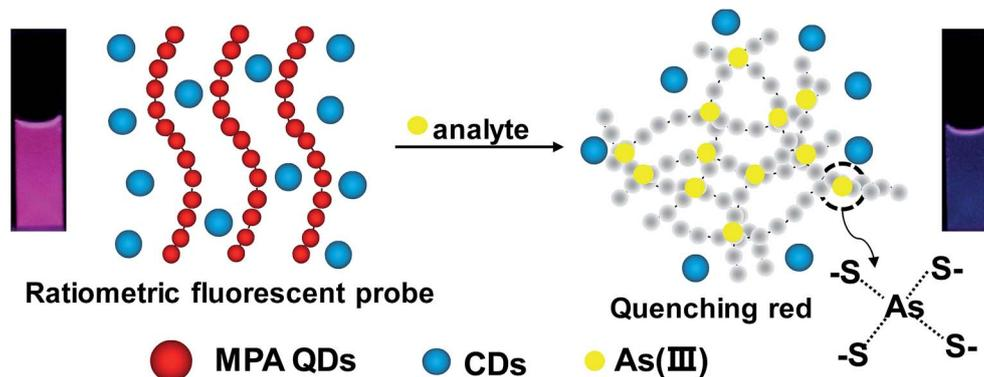
**Scheme 2** Schematic illustration of the ratiometric fluorescent sensors for the detection of As(III), the insets show the corresponding fluorescent photo under 365 nm UV lamp from fushia (left) to blue (right) upon the addition of As<sup>3+</sup> in the sensing system.
