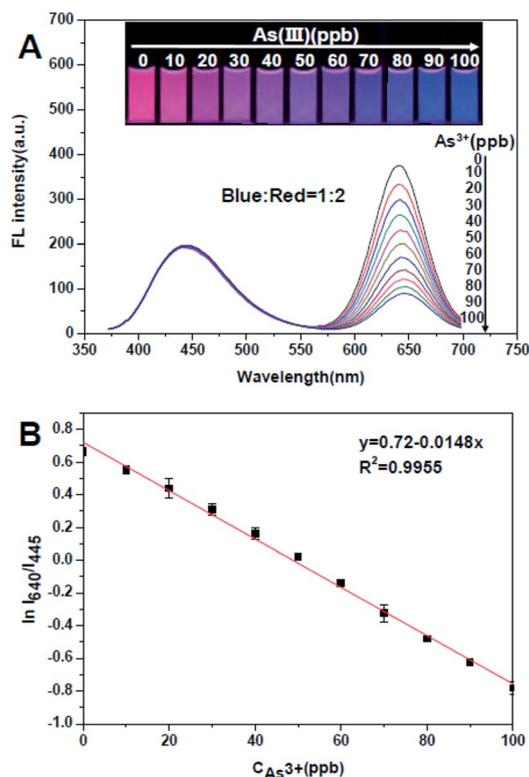
**Fig. 2** (A) The fluorescent spectra of mixture of blue CDs and red QD chains at ratios 1 : 2 with the addition of As(III). The insets show the corresponding fluorescent photo under 365 nm UV lamp. (B) Fluorescent intensity ratio,  $\ln(I_{640}/I_{445})$ , vs. the concentrations of As(III) in the TTCA-QD chains/CDs.
