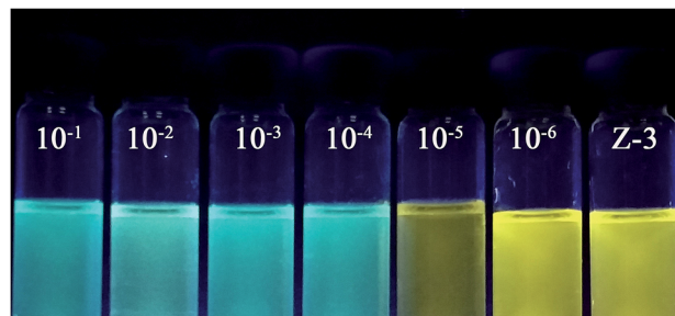
Fig. 6 Naked-eyes detection limit under UV lamp at 365 nm. From left to right, the concentration of Hg 2+ is 10^{-1} M, 10^{-2} M, 10^{-3} M, 10^{-4} M, 10^{-5} M, 10^{-6} and 0 M.
