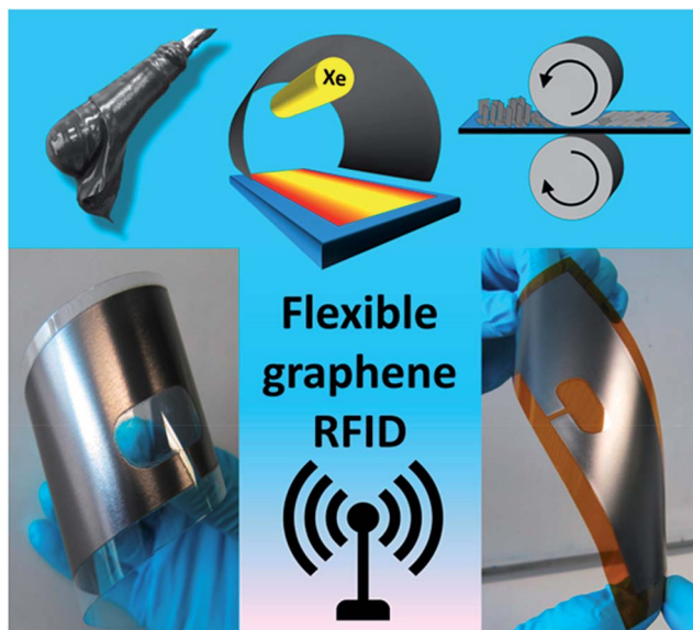
Fig. 11 Screen-printing and post-processing of graphene RFID antennas on flexible substrates including (left bottom) polyethylene terephthalate (PET), (right bottom) polyimide (PI). [Reprinted with permission from ref. 192 Copyright © Wiley.]
