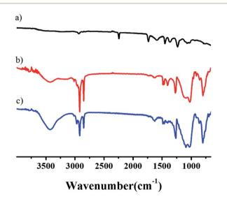
Fig. 2 FTIR spectra of aerogels at the following compositions: (a) fibers, (b) aerogel with fiber content is 0.3%, (c) the unmodified aerogel.
