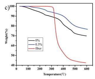
Fig. 3 The contact angles of unmodified (a) and modified aerogels (b). TG curves of aerogels with different fiber contents and fiber (c).
