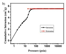
Fig. 4 Pore size distribution of the aerogel with 0.3% fibers (a) and the cumulative intrusion as a function of pressure (b).
