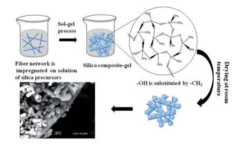
Schematic for the synthesis of silica aerogels.
