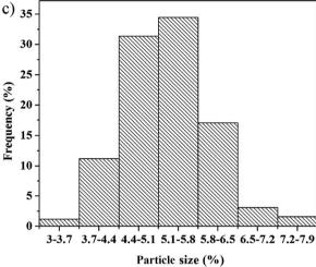
Fig. 1 SEM images of the aerogel with 0.3% fibers at different magnifications (a and b) and the particle size distribution of aerogel (c).
