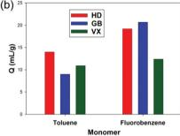
Fig. 5 (a) Before and after swelling of the fluorobenzene derived HCP against CWAs; HD, GB, and VX. (b) Swellability (Q) for the toluene and fluorobenzene derived HCPs against the three CWAs.
