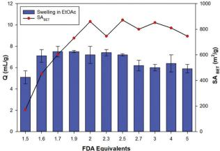
Fig. 3 Variation of the apparent BET surface area (SABET) and swellability (Q) in ethyl acetate, for the toluene derived HCPs.
