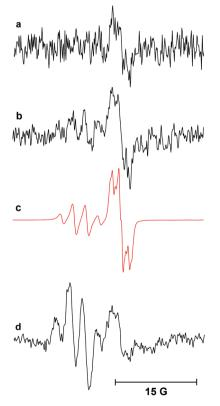
Fig. 1 EPR spectra during continuous photolysis of a solution of dihydropyridinone 6 in t-BuPh at 295 K. (a) 1 scan after 1 min UV irradiation. (b) 40 scans after 15 min UV irradiation. (c) Computed simulation. (d) 70 scans after 60 min UV irradiation.
