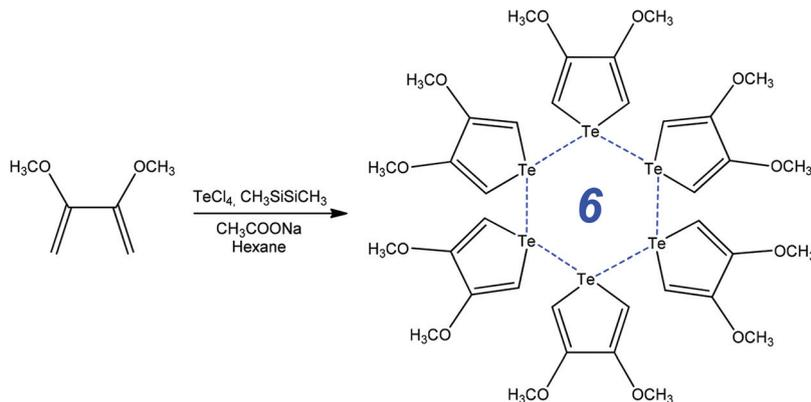
Scheme 8 Synthesis of 3,4-dimethoxytellurophene.<sup>80</sup>
