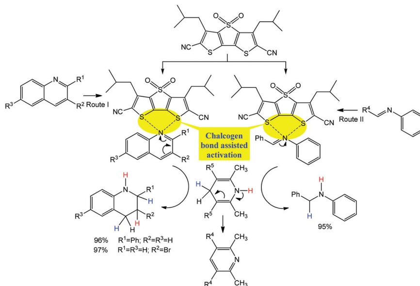
Scheme 18 Chalcogen bond assisted hydrogenation of quinolines (Route I) and imines (Route II).<sup>71</sup>
