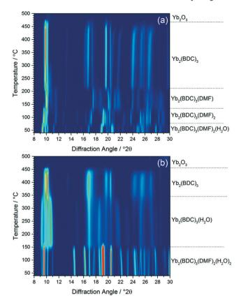
Fig. 5 In situ XRD measured (a) (1) and (b) (2) on heating in air, with assignment of each phase present based on TGA (see ESI†).
