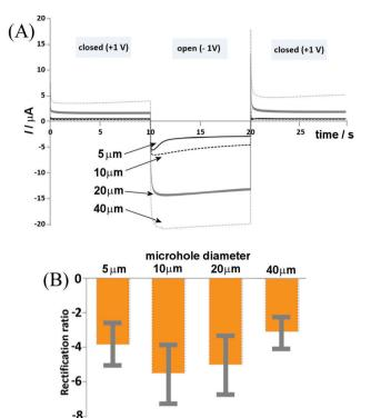
Fig. 7 (A) Chronoamperometry transient data for chitosan-doped cellulose film diodes switching between +1 V (closed state) and -1 V (open state) for PET microholes of 5, 10, 20, and 40 µm diameter immersed in 50 mM NaCl. (B) Bar plot of rectification ratios as a function of microhole diameter. Errors are estimated as ±30% to account for some variations in the film formation
