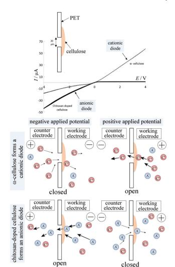
Fig. 5 Cyclic voltammetry (scan rate: 20 mV s $^{-1}$ ) of  $\alpha$ -cellulose only films (dotted line) and chitosan-doped cellulose films (black solid line) on a 20  $\mu$ m diameter microhole in a PET sheet in 50 mM NaCl on both sides of the membrane. The schematic drawing shows the four mechanistic cases of a cationic diode and an anionic diode under positive potential and negative potential polarisation, respectively.
