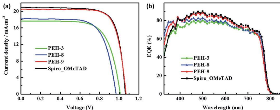
Fig. 5 (a) Current ( $J$ )–voltage ( $V$ ) curves of the solar cells with PEH-3, PEH-8, PEH-9 and Spiro-OMeTAD control recorded from forward bias (FB) to short circuit conditions (SC) under AM 1.5 conditions ( $100 \text{ mW cm}^{-2}$ ). (b) Incident photon-to-electron conversion efficiency (IPCE) as a function of wavelength for the PSCs in (a).
