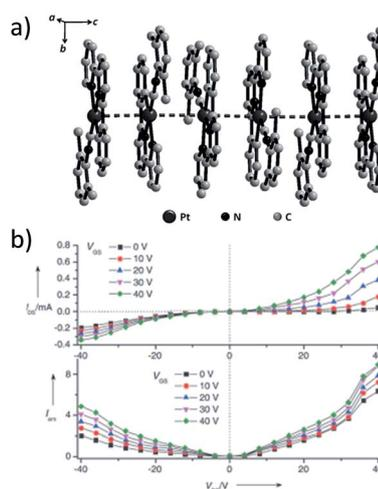
Fig. 9 (a) Crystal packing diagram of **61**· $\text{H}_2\text{O}$ . The  $\text{PF}_6^-$  and water molecules are omitted for clarity. (b) Output characteristics ( $I_{\text{DS}}$  vs.  $V_{\text{DS}}$ ) and electroluminescence intensity ( $I$ ) of an OLEFET device with nanowires of **61** after annealing at 350 K (adapted with permission from ref. 112. Copyright 2008, Wiley-VCH Verlag GmbH & Co. KGaA).
