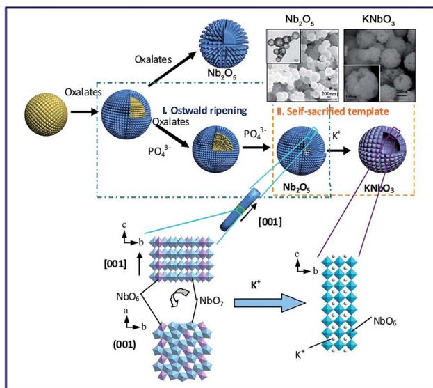
Fig. 4 Formation processes and structure evolution of the  $\text{KNbO}_3$  hollow spheres and  $\text{Nb}_2\text{O}_5$  solid spheres. The insets are the  $\text{Nb}_2\text{O}_5$  hollow spheres and the  $\text{KNbO}_3$  hollow spheres (ref. 31 Copyright 2013, the Royal Society of Chemistry).
