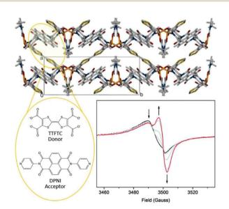
Fig. 3 The charge transfer MOF [(Zn(DMF))<sub>2</sub>(TTFTC)(DPNI)] which exhibits through-space CT interactions. Reduction of the MOF switches the CT off. This is consistent with solid state EPR spectroelectrochemistry which revealed evidence for a concomitant decrease in the TTFTC radical cation. and an increase in the DPNI radical anion signal, thus reducing the donoracceptor interaction. Reproduced from ref. 62 with permission from the Royal Society of Chemistry.
