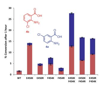
Fig. 3 The % conversion of anthranilic 4, by PrnA mutants, and ratios of products 5- and 3-chloroanthranilic acid ( $4a \div 4b$ ) after 1 hour with halogenase enzyme ( $10 \mu M$ ) and substrate (0.5 m M).
