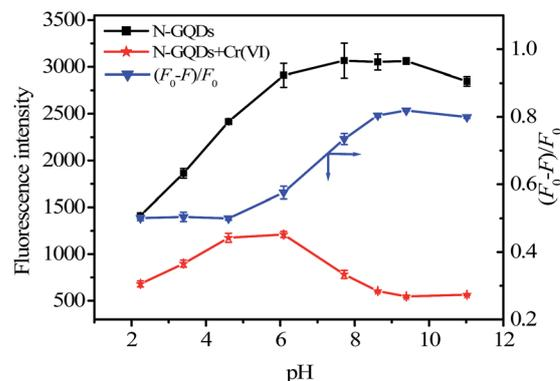
Fig. 3 FL responses of  $52\text{ mg L}^{-1}$  N-GQDs at 430 nm in the absence (black triangle) and presence (black square) of  $140\text{ }\mu\text{M}$  Cr(vi) ions at different pH values. Relative FL intensities  $[(F_0 - F)/F_0]$  at 430 nm of solutions of N-GQDs in the presence (blue) of  $140\text{ }\mu\text{M}$  Cr(vi) ions at different pH values.
