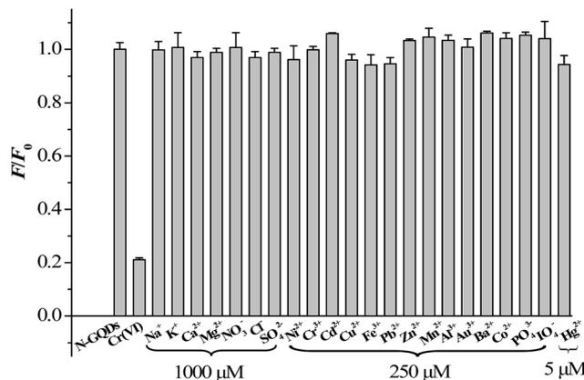
Fig. 6 Relative fluorescence intensities  $F/F_0$  at 430 nm of the N-GQDs solution after addition of 140 μM Cr(vi) and various other ions at 5 to 1000 μM.
