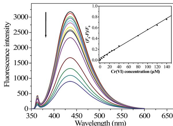
Fig. 5 FL response of 52 mg L<sup>-1</sup> N-GQDs upon addition of different concentrations of Cr(vi) ions solution. The arrows indicate the signal changes as increases in analyte concentrations (0, 1, 4, 8, 10, 15, 20, 25, 30, 40, 80, 120, and 140 μM). Inset: plot of the values of  $(F_0 - F)/F_0$  at 430 nm versus the concentrations of Cr(vi). The error bars denote standard deviations based on three independent measurements.
