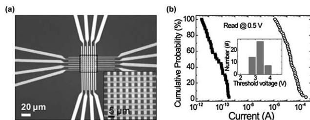
**Fig. 19** (a) An optical image of a 2  $\mu\text{m}$ -scale memory device in an 8  $\times$  8 array structure. (b) A  $I$ – $V$  curve of the 100 nm-scale device. Reproduced with permission.<sup>26</sup> Copyright 2011, Wiley.
