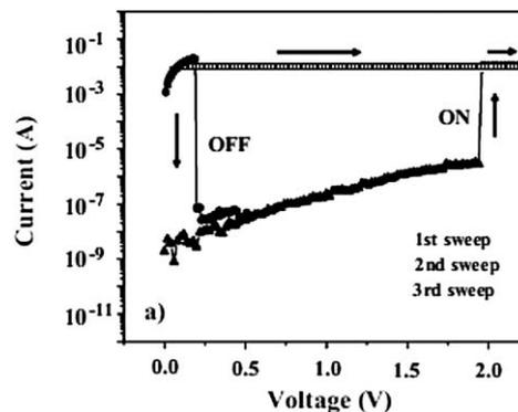
**Fig. 16**  $I$ - $V$  curves of 6F-HAB-CBZ PI. The current compliance of the first and second sweeps were set to 0.01 A, while the third sweep was set to 0.1 A. Reproduced with permission.<sup>7</sup> Copyright 2008, Wiley.
