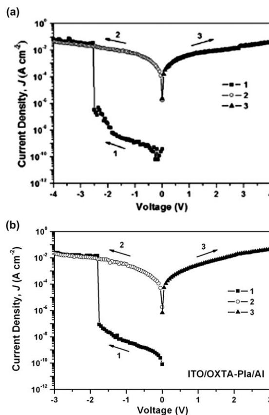
**Fig. 6**  $J$ – $V$  curves of (a) AZTA-PIa and (b) OXTA-PIa. Reprinted with permission from ref. 18 and 20. Copyright 2010, American Chemical Society,<sup>18</sup> Wiley.<sup>20</sup>
