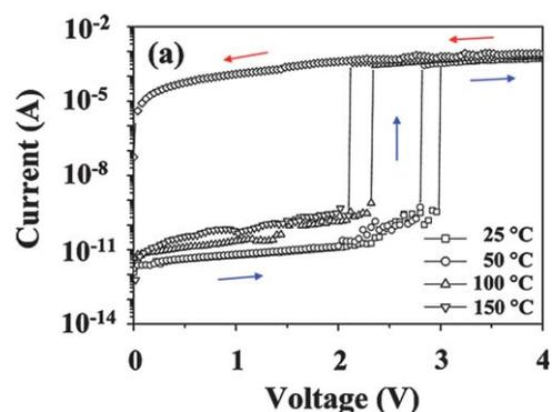
**Fig. 15**  $I$ - $V$  curves measured for the ITO/6F-HTAP PI/Al device at various temperatures under a nitrogen atmosphere. Reprinted with permission from ref. 15. Copyright 2009, American Chemical Society.
