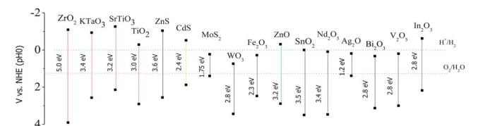
Fig. 3 Band edge position of several semiconductors, using the normal hydrogen electrode (NHE) as a reference (adapted with permission from ref. 23, copyright 2009 Royal Society of Chemistry).
