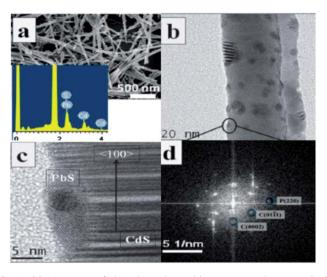
**Fig. 8** (a) SEM image of PbS/CdS synthesized by a cation exchange method, inset is EDX of the heterostructure. (b) TEM image showing a section of the nanowire with islands. (c) HRTEM indicating the presence of CdS and (d) FFT (SAED) pattern confirming the formation of PbS (reprinted with permission from ref. 69, copyright 2012 Royal Society of Chemistry).
