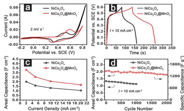
**Fig. 4** (a) CV curves, (b) CP plots, (c) areal capacitances and (d) capacitance as a function of cycle number for NiCo<sub>2</sub>O<sub>4</sub> NW arrays and hierarchical NiCo<sub>2</sub>O<sub>4</sub>@MnO<sub>2</sub> core-shell NW arrays on Ni foam.
