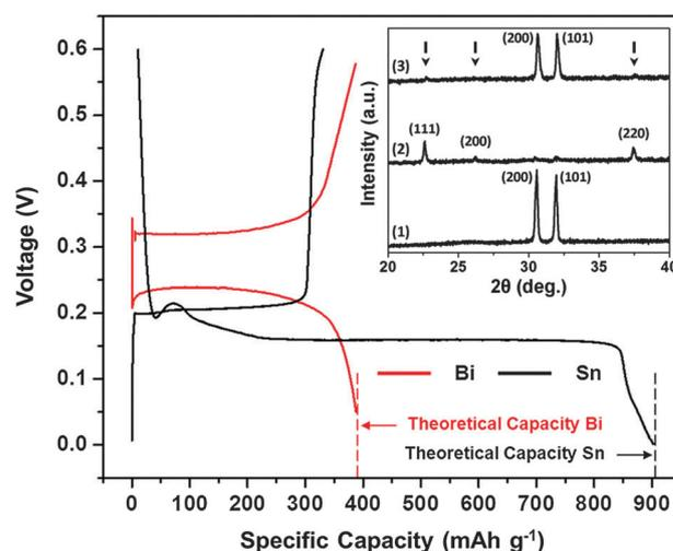
**Fig. 1** 1st cycle galvanostatic magnesiation/de-magnesiation curves for Sn/Mg (black) and Bi/Mg (red) half-cells (using organohaloaluminate electrolyte) highlighting their achievable theoretical capacities. Inset – XRD spectra for (1) as-fabricated Sn, (2) magnesiated Sn (or Mg<sub>2</sub>Sn – peak positions marked with arrows) and (3) de-magnesiated Mg<sub>2</sub>Sn.
