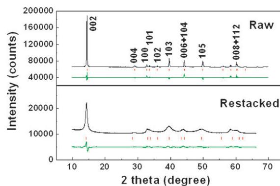
**Fig. 2** Rietveld refinement of XRD patterns of raw (top) and restacked (bottom) MoS<sub>2</sub>. The observed pattern, the calculated peak positions, and the difference between the observed and the calculated patterns are shown in black, red and green, respectively, from top to bottom.
