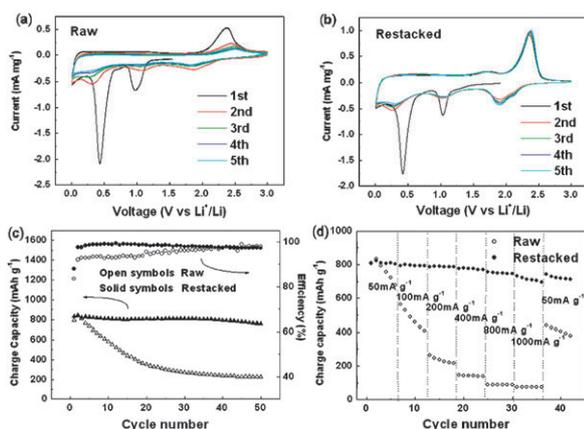
**Fig. 3** Electrochemical properties of raw and restacked MoS<sub>2</sub>: cyclic voltammograms of (a) raw and (b) restacked MoS<sub>2</sub> at a scanning rate of 0.2 mV s<sup>-1</sup>; (c) cycling performances at a current density of 50 mA g<sup>-1</sup>; (d) rate capabilities at different current densities (discharge current density was kept at 50 mA g<sup>-1</sup>).
