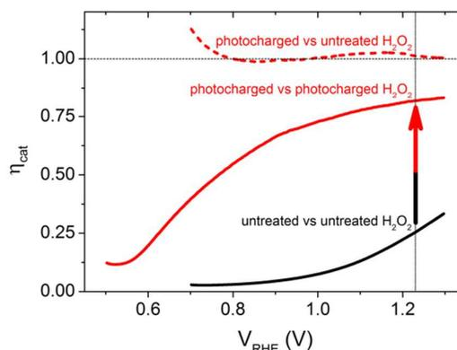
Figure 2 Calculated catalytic efficiency for the untreated (black solid curve) and photocharged  $\text{BiVO}_4$  samples (red curves). The catalytic efficiency for the photocharged samples was estimated using the JV characteristics in the presence of  $\text{H}_2\text{O}_2$  for the untreated sample (dashed red curve) and with the photocharged sample (solid red curve).
