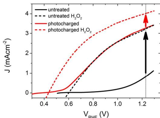
Figure 1 J-V scans of 200 nm thick  $\text{BiVO}_4$  under back-side AM1.5 illumination, in 0.1 M K-Pi buffer (pH 7.2), scan rate  $50 \text{ mVs}^{-1}$ , anodic sweeps. Arrows denote catalytic limitations for untreated (black) and photocharged (red) material.
