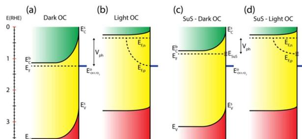
Figure 3 Estimated electronic band diagrams for  $\text{BiVO}_4$  in the OC configuration without surface states present (a) in the dark and (b) under illumination, and with surface states present (c) in the dark, and (d) under illumination.
