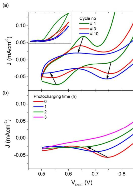
Figure 6 JV scans under illumination, for (a) untreated BiVO<sub>4</sub>, inset: full potential range, and (b) BiVO<sub>4</sub> photocharged for different periods of time (cathodic sweeps only).
