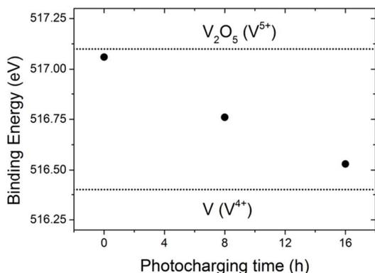
Figure 7 (a) XPS spectra for BiVO<sub>4</sub> photoanodes photocharged for 0 (black), 8 (red) and 16 h (blue) in K-Pi buffer pH 7.2. (b) V2p<sub>3/2</sub> peak position for BiVO<sub>4</sub> samples photocharged for different amount of time. V<sub>2</sub>O<sub>5</sub> and V(IV) binding energies are shown for reference.
