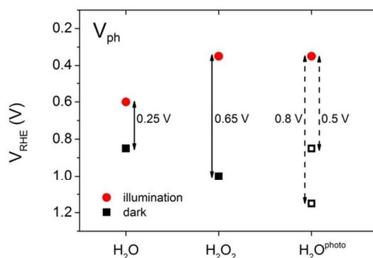
Figure 4 Equilibrium potentials and photovoltage values of  $\text{BiVO}_4$  photoanodes in the open circuit configuration: untreated sample in 0.1M K-Pi electrolyte ( $\text{H}_2\text{O}$ ), in presence of a hole scavenger ( $\text{H}_2\text{O}_2$ ), photocharged sample ( $\text{H}_2\text{O}^{\text{photo}}$ ).
