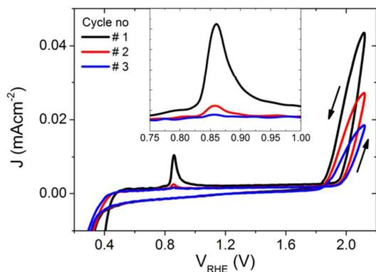
Figure 5 The first three dark JV scans of the BiVO<sub>4</sub> photoanode after 10 hours of photocharging, inset: a zoomed in plot around the observed oxidation peak at  $\sim 0.85 V_{RHE}$ .
