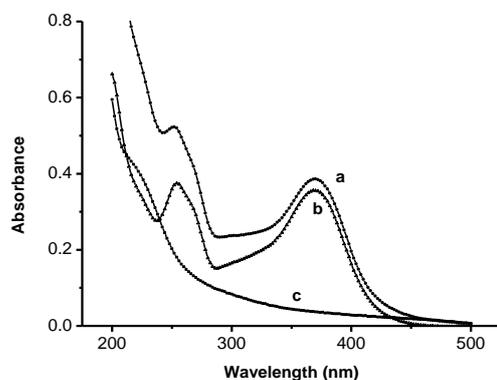
Fig.6 (B). The fluorescent intensity :aqueous CdSe/ZnS QDs (a); the aqueous CdSe/ZnS QDs-querctin solution system (b); the querctin(c). ( $C_{\text{querctin}}: 11.52 \text{ mg L}^{-1}$ ,  $C_{\text{CdSe/ZnS QDs}}: 1.2 \times 10^{-5} \text{ mol L}^{-1}$ ).
