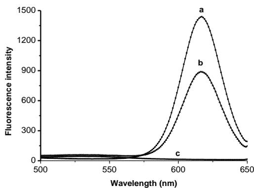
Fig.7. Fluorescence quenching of aqueous CdSe/ZnS QDs by adding different amount of querctin.
