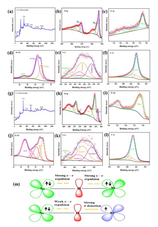
Fig. 5 High-resolution XPS spectra of (a and g) survey scan (b and h) Ni 2p, (c and i) Fe 2p, (d and j) Se 3d, (e and k) N 1s, (f and l) C 1s of  $Ni_xFe_{1-x}Se_2-NC@400$  and  $Ni_{3-x}Fe_xSe_4-NC@550$ , (m) schematic representation of electronic coupling of Ni-O-Fe in  $Ni_xFe_{1-x}Se_2-NC@400$ .
