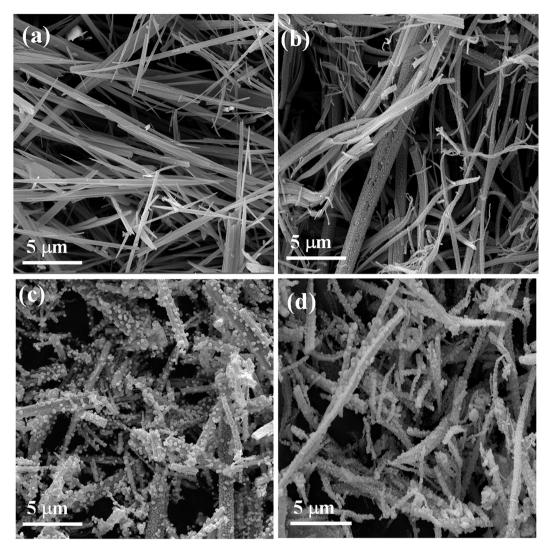
Fig. 3 FESEM images of (a) NiFe-NTA, (b) NiFe-NC@800, (c) Ni<sub>x</sub>Fe<sub>1-x</sub>Se<sub>2</sub>-NC@400, and (d) Ni<sub>3-x</sub>Fe<sub>x</sub>Se<sub>4</sub>-NC@550.
