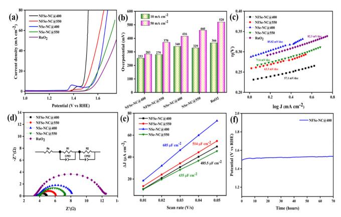
Fig. 6 (a) LSV curves, (b) required overpotential comparison at current densities 10 mA cm<sup>-2</sup> and 50 mA cm<sup>-2</sup>, (c) Tafel plots derived from amperometry, (d) corresponding Nyquist plots at 1.58 V vs. RHE (inset EIS Circuit), (e) capacitive current against scan rates on different electrocatalysts, and (f) chronopotentiometry measurement at the OER current density of 20 mA cm<sup>-2</sup> for NFSe–NC@400 electrode.
