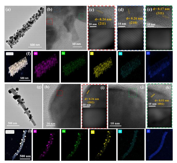
Fig. 4 (a) TEM, (b-e) HRTEM and inverse FFT of corresponding images, and (f) HAADF-elemental mapping images of Ni<sub>x</sub>Fe<sub>1-x</sub>Se<sub>2</sub>-NC@400, (g) TEM images, (h-k) HRTEM images and inverse FFT of corresponding images, and (l) HAADF-elemental mapping of Ni<sub>3-x</sub>Fe<sub>x</sub>Se<sub>4</sub>-NC@550.
