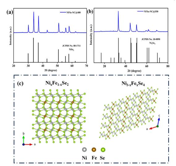
Fig. 2 XRD patterns of (a)  $Ni_xFe_{1-x}Se_2-NC@400$  and (b)  $Ni_{3-x}Fe_xSe_4-NC@550$  (c) crystal structure of  $Ni_xFe_{1-x}Se_2$  and  $Ni_{3-x}Fe_xSe_4$ .
