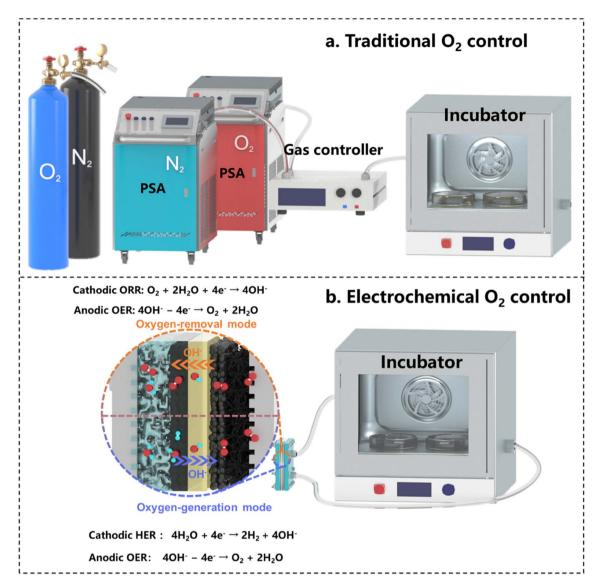
Working mechanisms of different  $O_2$ -control methods: (a) traditional  $O_2$ -control method, and (b) electrochemical  $O_2$ -control method.
