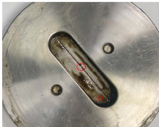
Fig. 10 The condition of the crack board in the plugging experiment of the crack width is 0.25\ \mu\text{m} .
