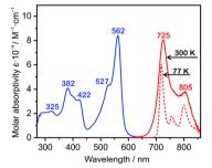
Fig. 7 Absorption and photoluminescence spectra of Pt-7 in toluene solution at 300 K and 77 K. Reproduced from ref. 39 with permission from the Royal Society of Chemistry.
