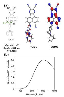
Fig. 19 (a) The HOMO and LUMO of CAT-1. (b) EL spectrum of the nondoped OLED fabricated with CAT-1. Adapted with permission from ref. 103 Copyright 2019 American Chemical Society.
