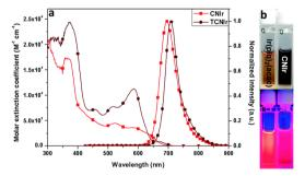
Fig. 14 (a) Absorption and photoluminescence spectra of complexes Ir-10 (light red lines) and Ir-11 (dark red lines) in tetrahydrofuran. (b) Solutions of Ir-10 (right) and reference complex Ir(pic)2(acac) (left) photographed in visible (top) and ultraviolet light (bottom). Reproduced from ref. 80 with permission from the Royal Society of Chemistry.
