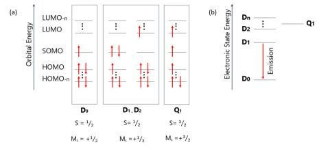
Fig. 26 (a) Molecular orbital diagrams for a doublet emitter showing electron occupancy in ground state  $(D_0)$  and excited states  $(D_1, D_2, \text{ and } Q_1)$ . (b) Jablonski energy diagrams of the doublet-quartet manifold, indicating doublet-doublet fluorescence. Adapted from ref. 152, with the permission of AIP Publishing
