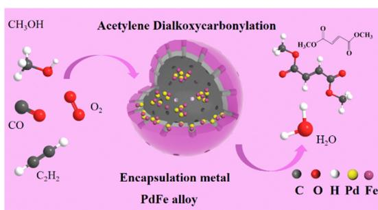
**High activity nitrogen-doped hollow carbon/silicon hollow spheres as encapsulated Pd–Fe nano-reactors for acetylene dialkoxy carbonylation**
