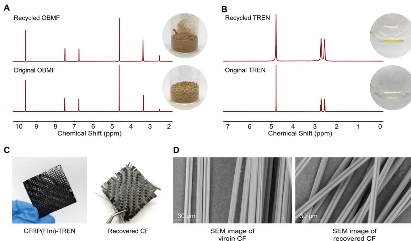
**Fig. 2** Chemical recycling of P(FIm)-TREN: physical appearance and <sup>1</sup>H NMR spectra of OBMF in DMSO-*d*<sub>6</sub> (A) and TREN in D<sub>2</sub>O (B) after depolymerization and subsequent purification, visual appearance of CFRP(FIm)-TREN and recovered carbon fiber cloth upon depolymerization of the composite (C), SEM images of virgin and recovered carbon fibers (D). Scale bar is 30 μm.
