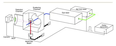
Fig. 1 Schematic illustration of the NAP-VMI apparatus.
