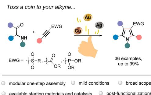
**Coinage (Au, Ag, Cu) metal-catalyzed (3 + 2) annulation of  $\alpha$ -aminoketones and electron-deficient alkynes as a route to 3-EWG-substituted pyrroles**
