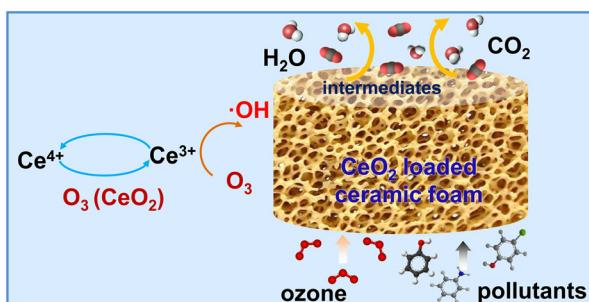
**CeO<sub>2</sub>-modified monolithic ceramic foams for efficient catalytic ozonation of refractory organic pollutants in a continuous-flow reactor**
