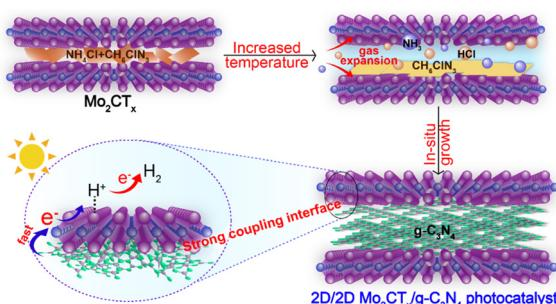
**2D/2D  $\text{Mo}_2\text{CT}_x/\text{g-C}_3\text{N}_4$  with a strong coupling interface via one-step  $\text{NH}_4\text{Cl}$ -assisted calcination for enhanced photocatalytic hydrogen production**
