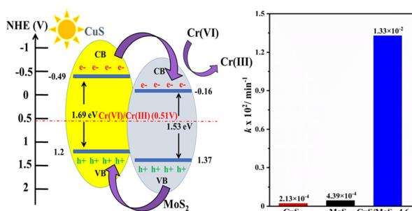
**Construction of visible light active  $\text{CuS}/\text{MoS}_2$  heterojunctions for heightened photoreduction of Cr(vi)**
