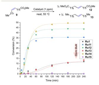
Scheme 3 Self-metathesis of methyl oleate (9, 95% pure). Conversion =  $100 \times [1 - (A_9 \times A_{1S}^0)/(A_9^0 \times A_{1S}^0)]$ ;  $A_{1S}^0$ ,  $A_{1S}^0$  = GC area of methyl oleate and internal standard before the reaction. Lines are visual aids only.
