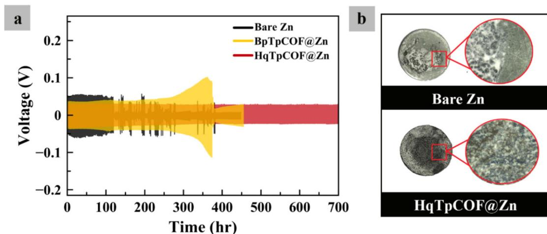
Fig. 4 (a) Long-term GCD profiles of the bare Zn electrode and COF layer coated on the Zn electrode at a current density of 1 mA cm<sup>-2</sup> and a capacity of 1 mA h cm<sup>-2</sup> and (b) surfaces of different electrodes after battery failure.
