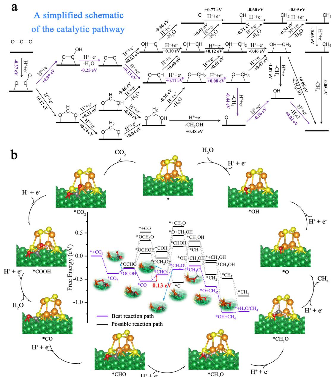
**Fig. 6** The CO<sub>2</sub>RR pathways on Ni100–Fe<sub>4</sub>S<sub>4</sub>. (a) A simplified schematic of the free energy changes ( $\Delta G$ ) in the entire possible CO<sub>2</sub>RR pathways; the energy optimal route is marked in purple. (b) The schematic diagram of the reaction mechanism of CO<sub>2</sub> electroreduction to CH<sub>4</sub> during the entire CO<sub>2</sub> reduction catalytic cycles.
