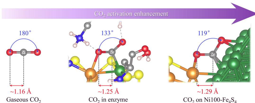
**Fig. 2** Schematic diagram of the geometric structure of CO<sub>2</sub> in different adsorption states and CO<sub>2</sub> activation enhancement. (In atomic coloring, white is H, gray is C, blue is N, red is O, yellow is S, orange is Fe, and green is Ni).
