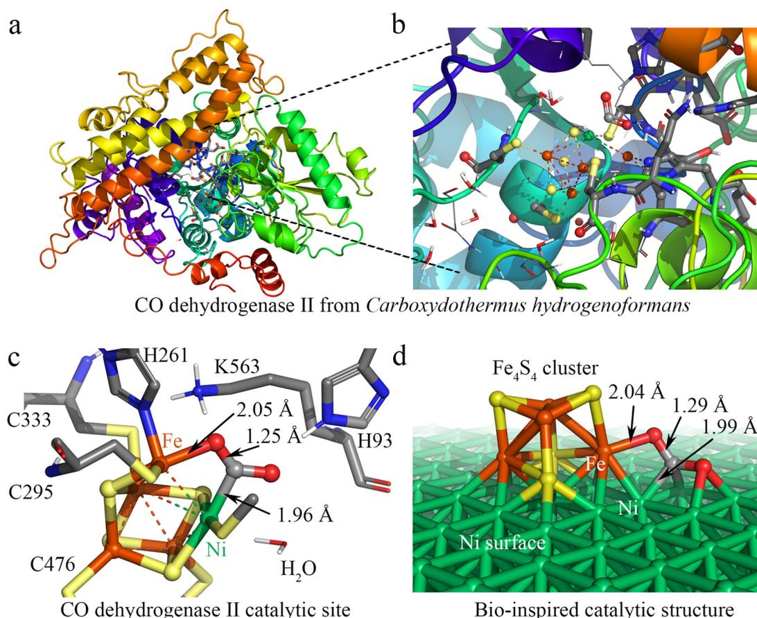
**Fig. 1** Design of the Ni100–Fe<sub>4</sub>S<sub>4</sub> catalyst inspired by CO dehydrogenase II. (a) The crystal structure of CODHII<sub>Ch</sub>. (b) The catalytic center of CODHII<sub>Ch</sub>. (c) The structure of the CODHII<sub>Ch</sub> catalytic center combined with CO<sub>2</sub>. (d) The structure of the bio-inspired heterogeneous Ni100–Fe<sub>4</sub>S<sub>4</sub> catalyst. (In atomic coloring, white is H, gray is C, blue is N, red is O, yellow is S, orange is Fe, and green is Ni).
