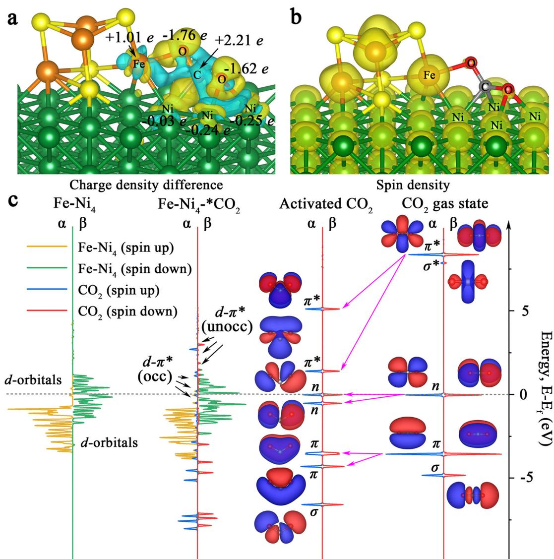
**Fig. 5** Associative and activation mechanism analysis. (a) Charge density difference of CO<sub>2</sub> adsorption on Ni100-Fe<sub>4</sub>S<sub>4</sub> (Light blue stands for the outflow and yellow for the inflow of electrons.). (b) Spin density of Ni100-Fe<sub>4</sub>S<sub>4</sub> (Yellow stands for spin electrons.). (c) Projected electronic densities of states (PDOS) of FeNi<sub>4</sub>, CO<sub>2</sub> and their interactive configuration FeNi<sub>4</sub>-\*CO<sub>2</sub>.
