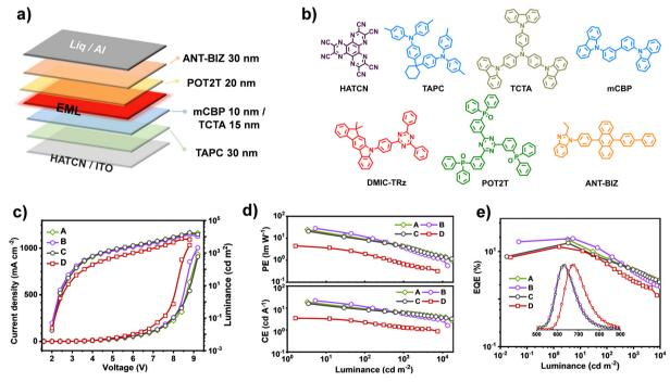
Fig. 5 (a) The diagram of OLED structures, and (b) chemical structures of the used materials. (c) The current density-voltage-luminance (J-V-L) curves of these devices. (d) Power efficiency and current efficiency as a function of luminance, and (e) EQE curves versus luminance, and EL spectra (inset, at the same driving voltage of 2.8 V) of these involved devices (A-D).
