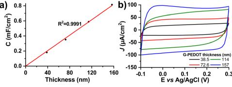
Fig. 3 Electrochemical capacitance of G-PEDOT. (a) Linear dependence of areal capacitance on the layer thickness. (b) Cyclic voltammograms (0.1 M KCl,  $100 \text{ mV s}^{-1}$ ) used for calculation of the capacitance.
