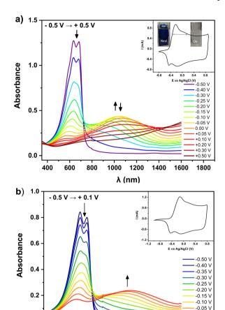
Fig. 2 CV scans and UV-vis-NIR spectra of thin films of G-PEDOT deposited on an ITO substrate, recorded for increasing electrode potential vs. Ag/AgCl pseudo-reference wire, under an inert atmosphere of argon. (a) Electrolyte: 0.1 M TBAPF<sub>6</sub>/CH<sub>3</sub>CN; (b) electrolyte: 0.1 M KCl/H<sub>2</sub>O.
