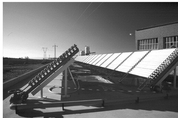
Fig. 22 One of the first pilot plants for photocatalysis, employing a slurry reactor (in a static concentrator array) installed at latitude 40° (Arganda del Rey, Madrid, Spain). Costing estimates in Section 1 for plant scale PCs are taken from this plant's operation. 62 Reproduced with permission from ref. 67. Copyright 2002 Elsevier B.V.
