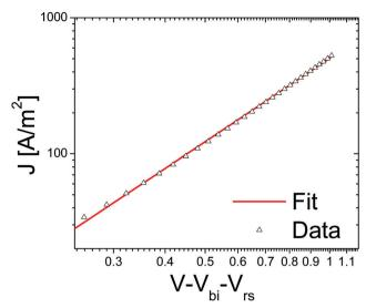
Fig. 6 Current density vs. voltage, corrected for built in voltage and series resistance of a bisPCBM electron only device. Data (symbols) is fitted (solid line) using a space charge limited current with a mobility of  $7 \times 10^{-8}$  m<sup>2</sup> V<sup>-1</sup> s<sup>-1</sup> (reprinted with permission from ref. 30. Copyright 2008 Wiley-VCH Verlag GmbH & Co. KGaA, Weinheim).
