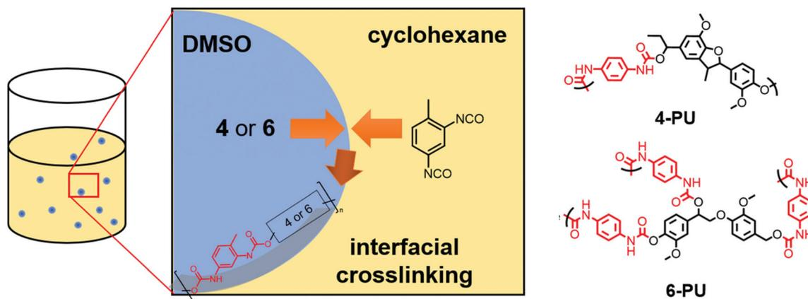
**Scheme 3** Scheme for the polyaddition reaction of phenylcoumaran **4** and  $\beta$ -O-4-aryl ether **6** with toluene diisocyanate (TDI) in an inverse mini-emulsion (DMSO : cyclohexane). **4** or **6** was dissolved in DMSO and dispersed in cyclohexane stabilized by the nonionic surfactant P(E/B-*b*-EO).
