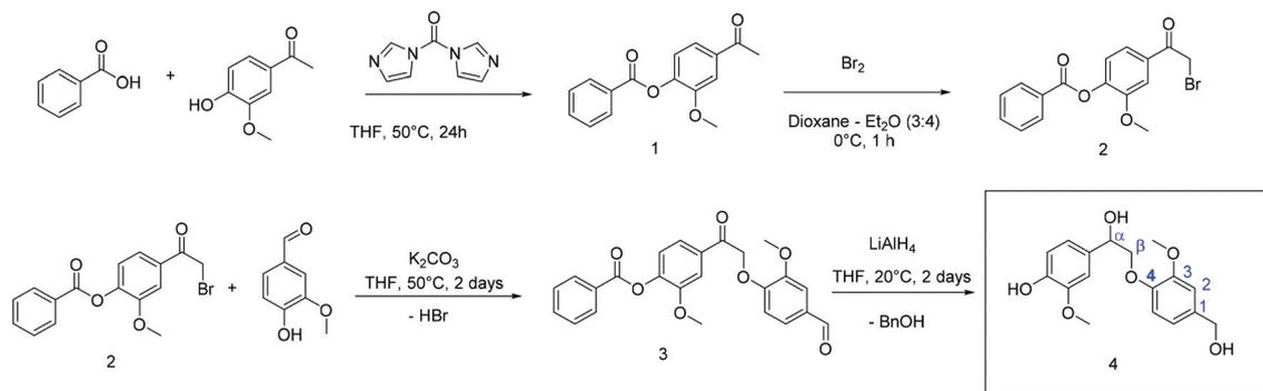
**Scheme 1** Synthesis of monomer **4** over four steps from bio-based acetovanillone and vanillin. The monomer is related to lignin's  $\beta$ -O-4-aryl ether binding motif, which is the most common linkage in lignin.
