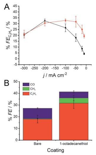
Fig. 4 (A) Faradaic efficiency for  $C_2H_4$  formation (%  $FE_{C_2H_4}$ ) during galvanostatic  $CO_2$  reduction at a 500 nm Cu GDE in 1 M KOH with (red) and without (black) a monolayer of 1-octadecanethiol to form a hydrophobic interface. (B) % FE for CO, CH<sub>4</sub> and  $C_2H_4$  with and without the 1-octadecanethiol layer during galvanostatic  $CO_2$  reduction at -50 mA cm<sup>-2</sup> using the same conditions as in (A). Error bars display one standard deviation (n=3).
