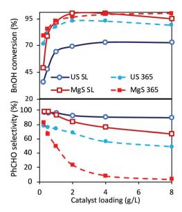
Fig. 3 BnOH conversion (up) and PhCHO selectivity (down) after 3 h for different catalyst loadings (0.5, 1, 2, 4 and 8 g  $L^{-1}$ ) under a US amplitude of 30% (US) or magnetic stirring (MgS) irradiating with solar light (SL) or ultraviolet light of 365 nm wavelength (365); the reported values are the average of three experiments with the error to be less than 1.5%.
