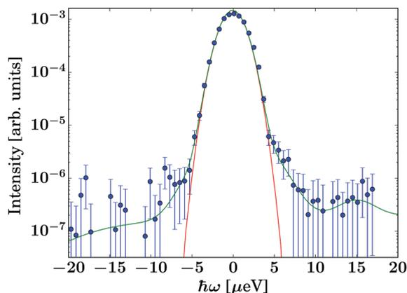
Fig. 2 Energy resolution function recorded at  $q = 1.08 \text{ \AA}^{-1}$  using a vanadium standard in the same geometry as the samples (symbols), and fit (green line), being well described by a Gaussian over 3 orders of magnitude (red line).
