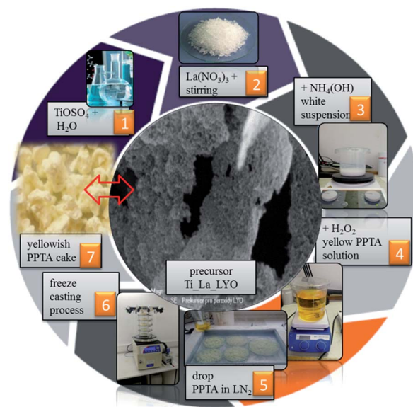
Scheme 1 Synthetic route for the preparation of [La(III)-peroxo-polytitanic acid] precursor \text{Ti}_{\text{La}}\text{LYO} .
