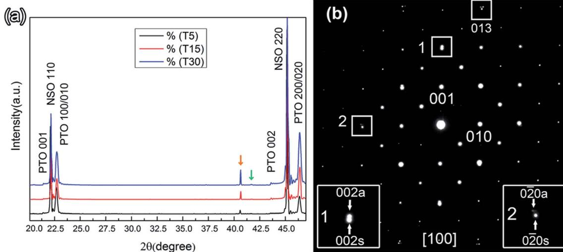
Fig. 1 (a) XRD  $\theta$ - $2\theta$  scan patterns of PTO thin films with different cooling rates grown on NSO substrates. Indexed peaks are K $\alpha$  of both NSO and PTO; the yellow and green vertical arrows indicate the K $\beta$  peaks of NSO 200 and PTO 200/020, respectively. (b) Selected area electron diffraction (SAED) pattern of the T5 PTO film on NSO substrate taken from the area including the film and substrate along [100] zone axis.
